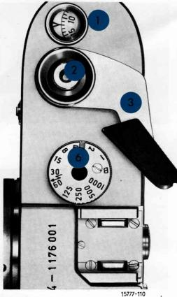
The film transport lever (3) simultaneously tensions the LEICA's focal-plane shutter and advances the film by one frame. Push the lever all the way to the right until a firm stop is felt. This can be done with a single thumb-stroke, or by a series of shorter strokes.
