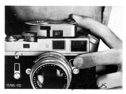
The 90mm focal frame built into the M 4 viewfinder system is therefore used, by means of the frame pre-selector (16), to give accurately aimed exposure readings. A LEICAMETER MR belongs on your LEICA M 4 because it lets you measure exactly what you want, and lets you know exactly what you are measuring.
